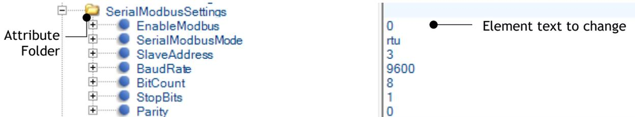
Figure 22: Expanded SerialModbusSettings Folder
