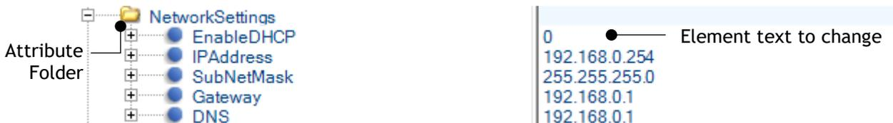
Figure 20: Expanded NetworkSettings Folder
