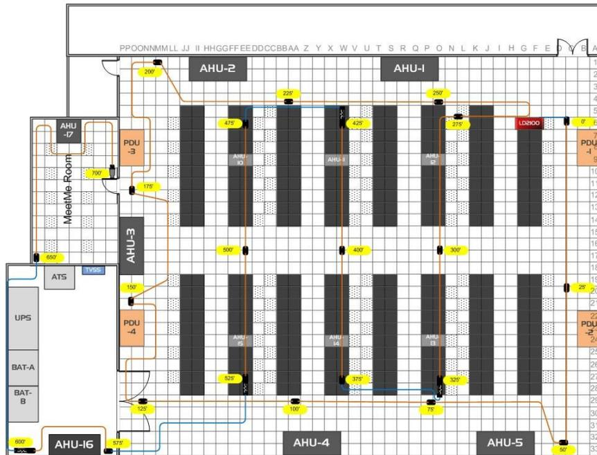
Figure 4.13 Leak Detection Reference Map
