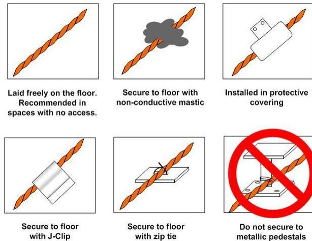
Figure 2.5 Secure the Cable
