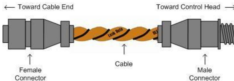
**Figure 2.4** Sensing Cable
