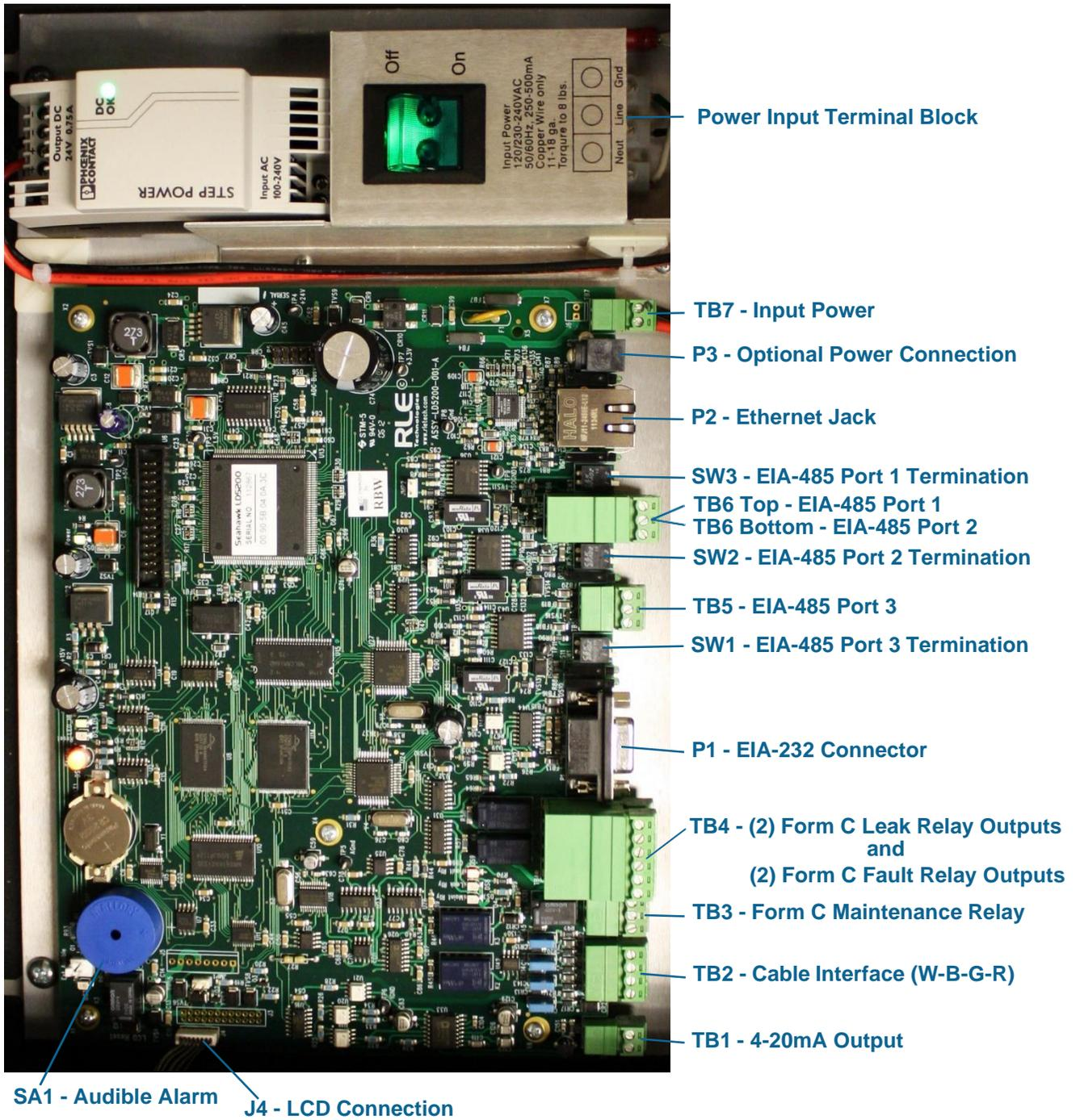
Figure 2.2 AQ5200 Physical Connections and Switches
