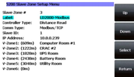
LCD - Slave Zone Setup Menu- Modbus
