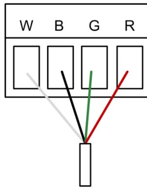
Figure 8 Cable connection TB2
