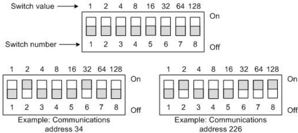
Figure 13 DIP Switch settings for Communications Address
