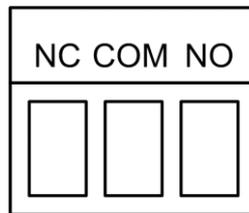
Figure 5 Relay Output Connection TB1
