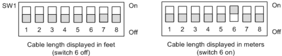
Figure 9 SW1, DIP Switch 6 - Display cable length in feet or meters
