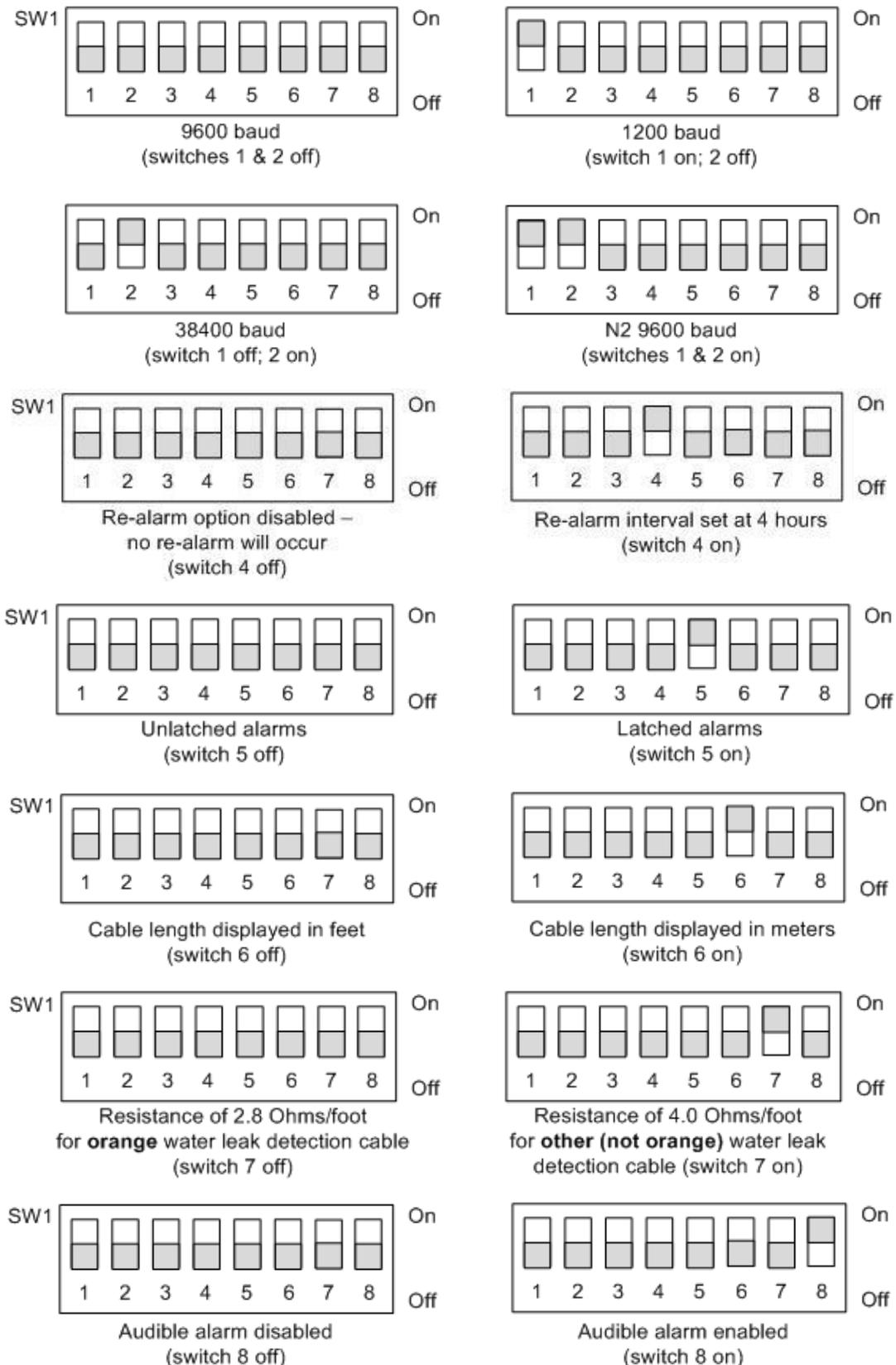
Figure A2 SW1 DIP Switch configuration settings
