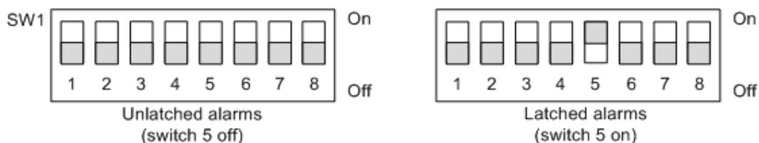
Figure 7 SW1, DIP Switch 5 - Latched or Unlatched Alarms
