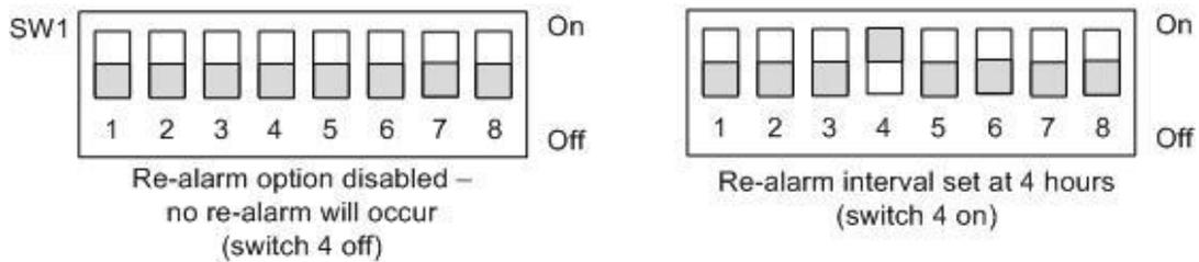
Figure 15 SW1, DIP Switch 4 - Re-Alarm interval
