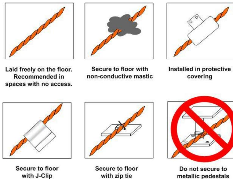
Figure 18 Securing the Sensor Cable
