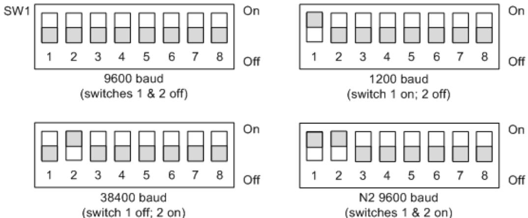
**Figure 12 DIP Switch settings for Communications Baud Rate**
