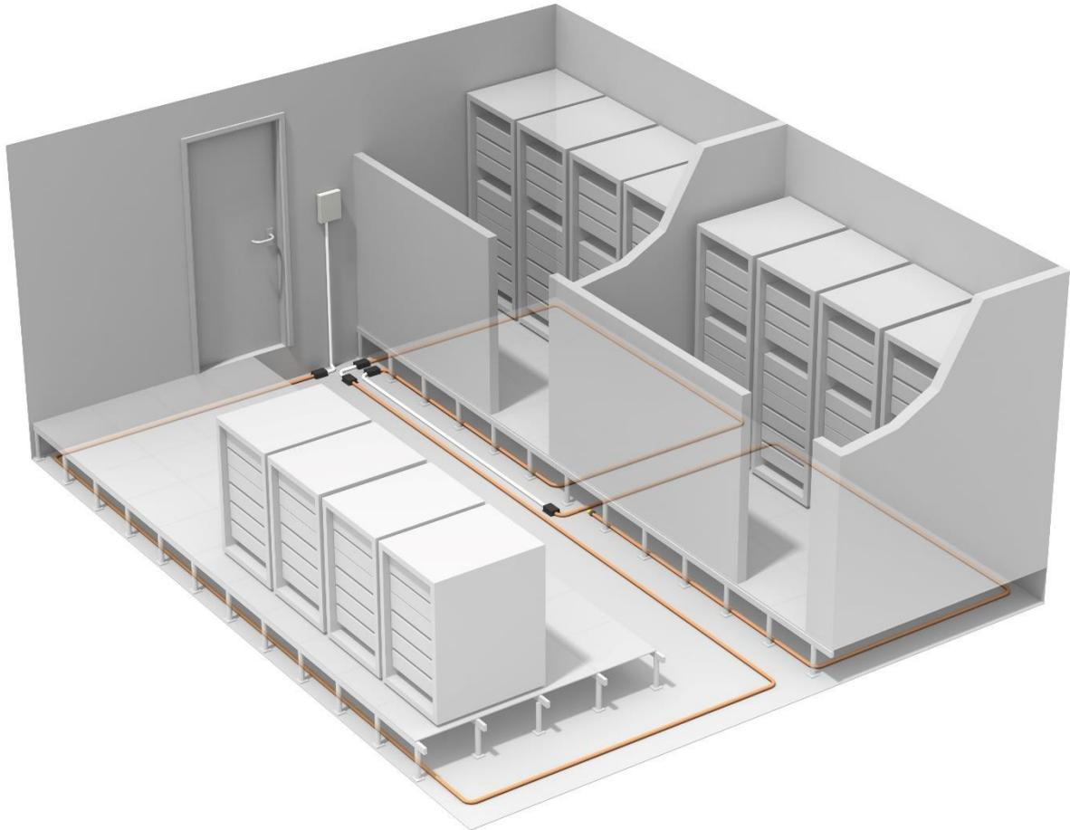
**Figure 17 Example of sensor cable routing in a large data centre**
