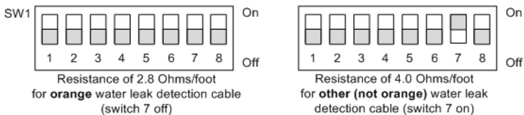
Figure 10 SW1, DIP Switch 7 - Ohms per foot resistance
