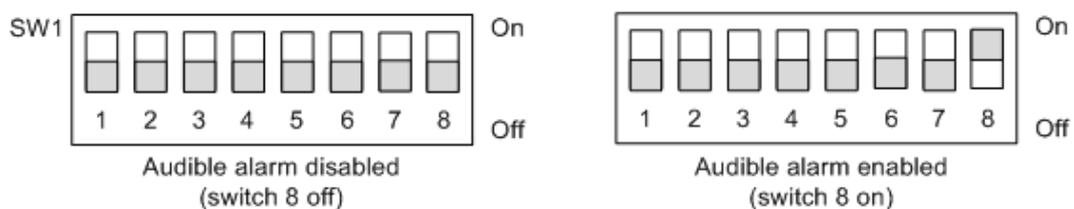
Figure 14 SW1, DIP Switch 8 - Audible Alarm settings
