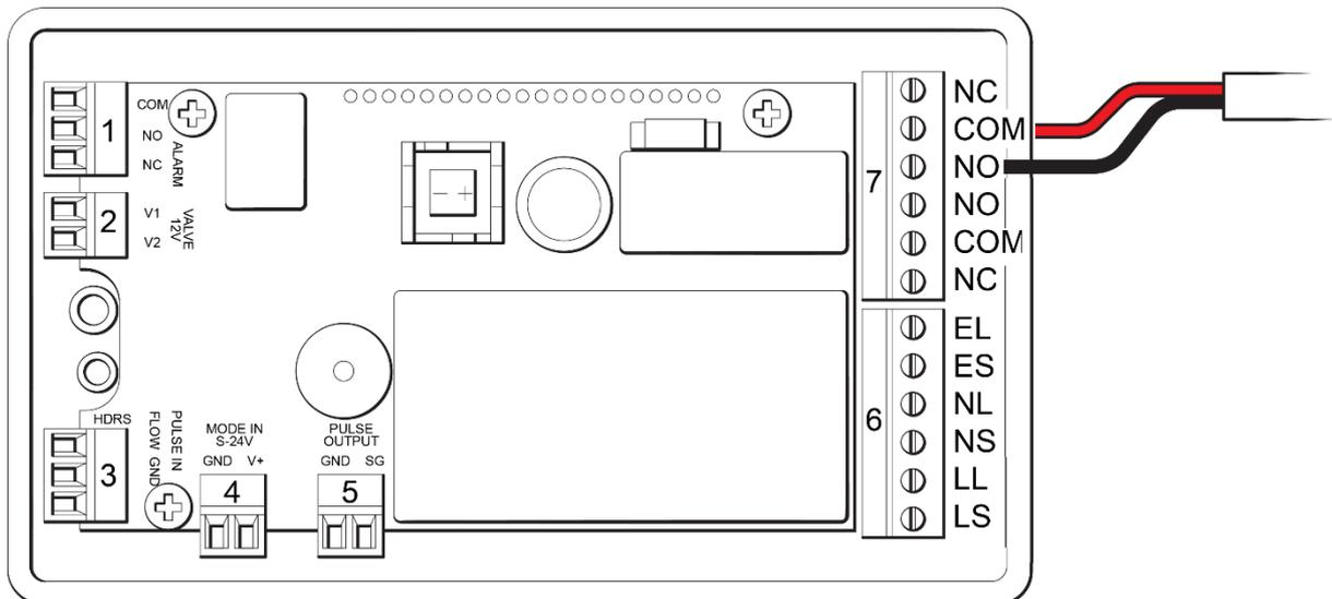
Figure 8. Normally Open (NO) Wiring Diagram for Beacon or SMS units
