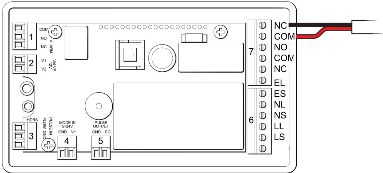
Figure 9. Normally Closed (NC) Wiring Diagram for Beacon or SMS units
