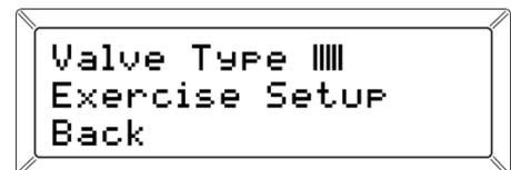
4. Use [+] and [-] to adjust the valve type in use. Press [Set] to save.
