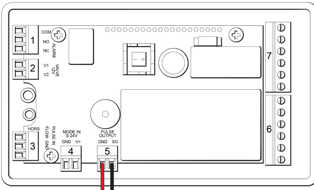
Figure 10. Wiring Diagram for Pulse Output to a Building Management System
