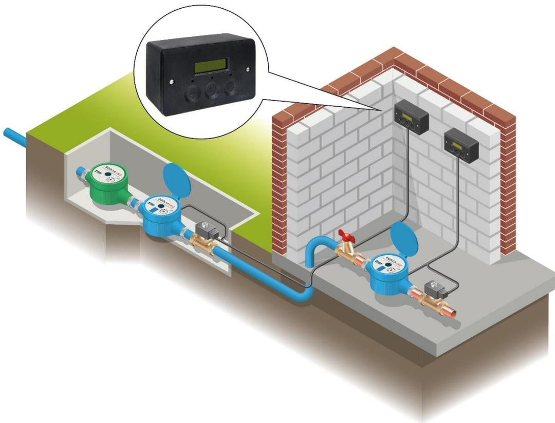
*Figure 3. External and Internal Configurations of Aqualeak WG Installation*
