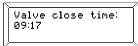
If the Monitoring Profile is set to Weekly, the valve transitions for each day assigned Period Schedule Mode must be programmed. It may be helpful to write this out prior to beginning. An example is given in Table 3.
