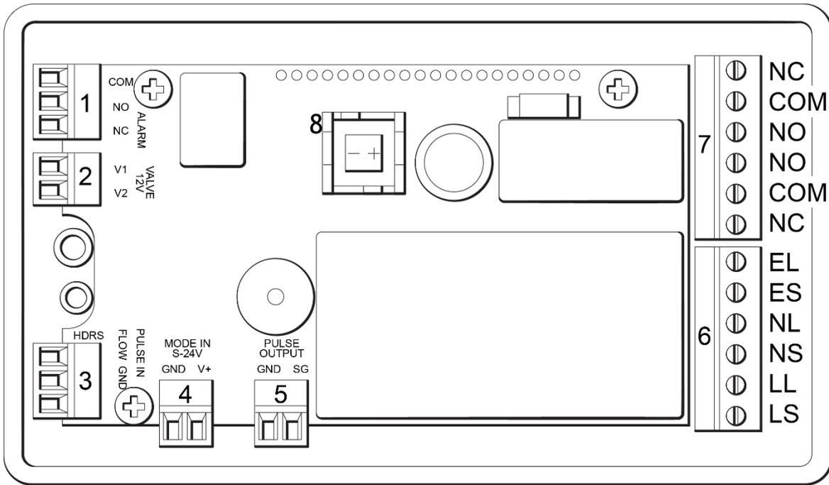
Figure 2: Aqualeak WG Input-Output Connections
