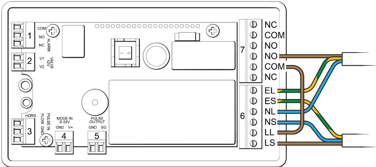
Figure 5. Normally Open (NO) Ancillary Wiring Diagram
