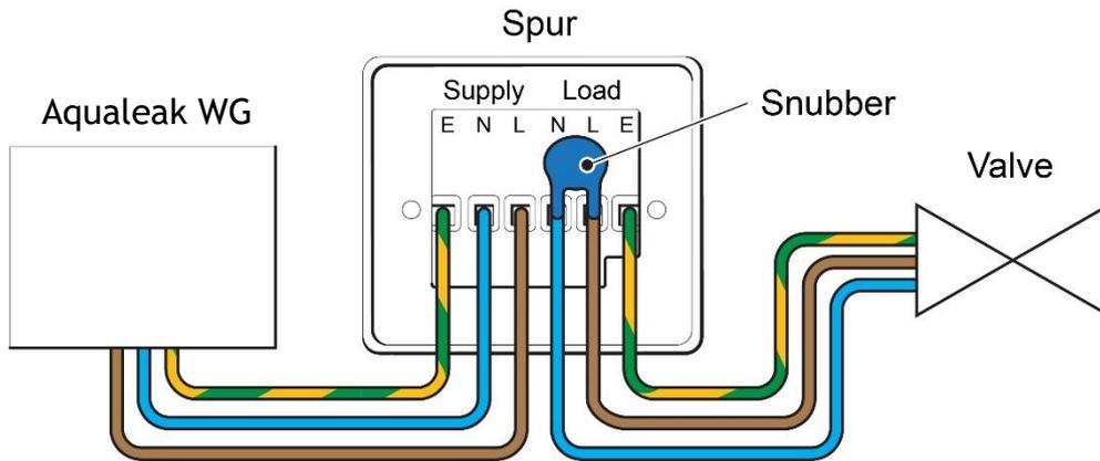
Figure 7. Snubber Wiring Diagram
