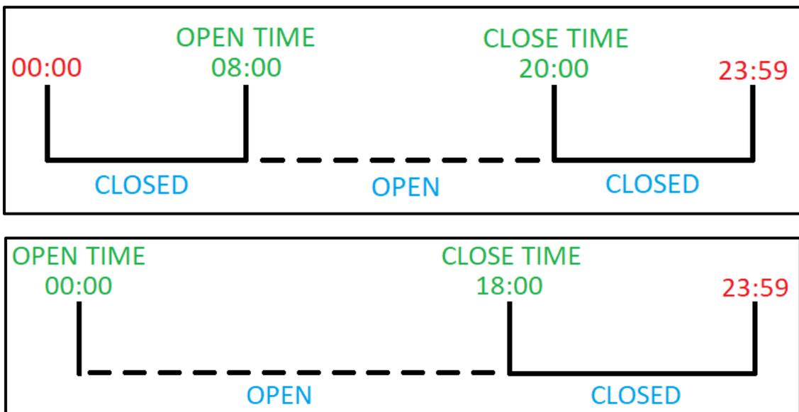
Figure 12. Examples of Scheduled Valve Programming
