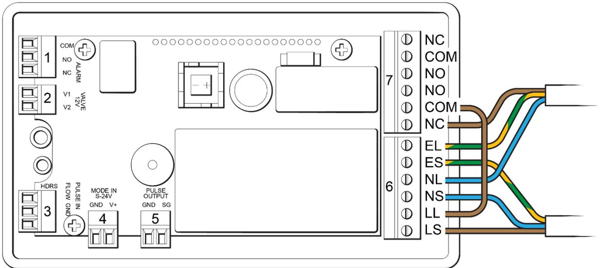
Figure 6. Normally Closed (NC) 230V Ancillary Wiring Diagram
